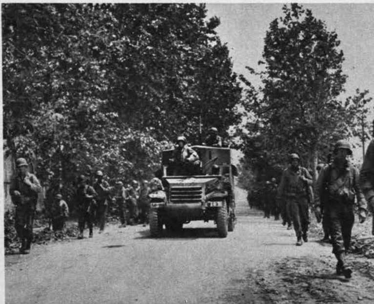
Earliest U.S. tank destroyer was the M-3 half-track with the old field artillery 75-mm. gun. Designated the M-3A1 gun carriage, this vehicle has an open driver's cab and carries a high shield for the gun crew.
